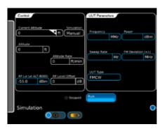
Simulated static altitude may be set by the user and manually incremented or decremented.
